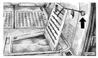
To open the main cover, pull up on the latch, and attach the cord to the rear seat head restraint post.
